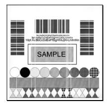
Streaks can indicate a dirty or faulty printhead.
