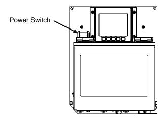
3. Connect the AC Power Cord to the printer and then to a properly grounded outlet.
