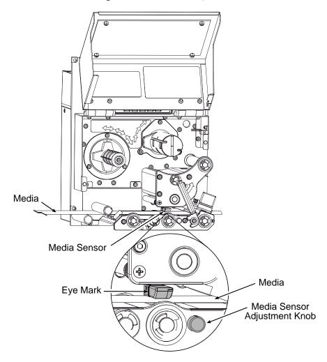
2. Depending on the type of media being used, rotate the Media Sensor Adjustment Knob until the Eye Mark on the Media Sensor is positioned according to the table below.
