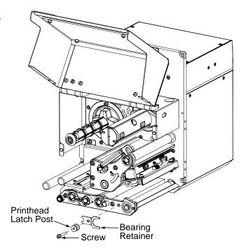
4. Remove the outer bearing and platen roller from the printer
