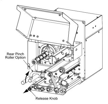
2. Route the Media between the Media Posts, through the Media Sensor, over the Peel Bar, and out of the printer, as shown below.
