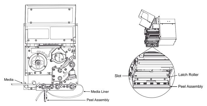
5. Pull the Media Liner through the Slot in the Peel Assembly until all slack is removed. Lifting from the center, raise the Peel Assembly until it locks into place.
