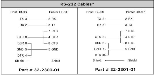
\*Printer serial ports A & C require a DB9 male connector (e.g., Startech C9PSM).
