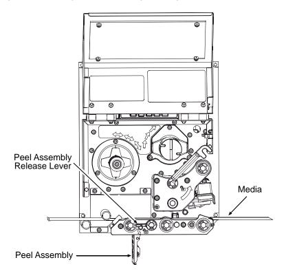
4. Remove the labels from 12 inches (30 cm) of the Media Liner. Route the Media Liner down to the Peel Assembly, over the Latch Roller, and through the Slot as shown below.
