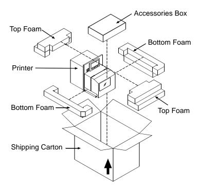
3. Remove the Printer from the plastic bag and then remove all remaining packing materials.
