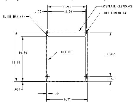
Attach the printer to the support structure using a #10 screw inserted at each Mounting Hole position (see note below).
